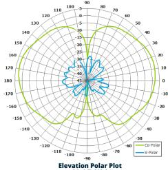
Elevation Polar Plot (@ 4.7 GHz)
